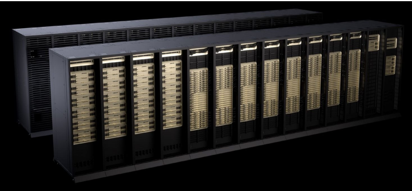
Figure 5. NVIDIA DGX Vera Rubin NVL72. Each rack connects 72 Rubin GPUs and 36 Vera CPUs in a single NVLink domain. Cortex deploys eight. Source: NVIDIA DGX Vera Rubin NVL72 datasheet.
