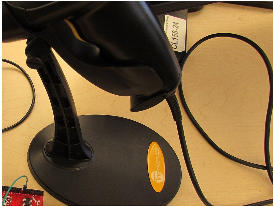
Figure 4. Capture hardware. A handheld scanner covers moves away from a station. Fixed barcode and RFID readers sit where material already stops: receiving, stock, production, packing.
